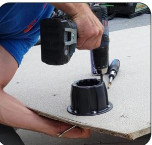
**18.** Replace the boat floor by lining up the bolts in the holes. Then put back all the floor screws.
