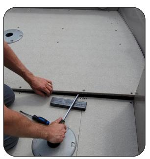
**6.** Make sure there are no electric wires, fuel tank, hoses, or any other critical parts underneath. Be sure that there is enough space between floor and hull to avoid damage it during drilling.
