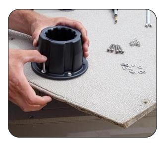
**16.** Underneath, put on each bolt a flat washer and a nylon nut.
