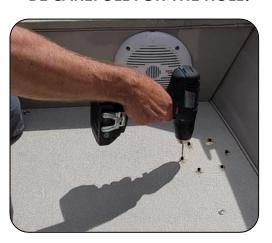
**11.** Clean the surface of drilling residue and position the base. Respect the order of the image below: **1. Screw, 2. Self-locking washer and 3. Flat washer.** Partially tighten the 6 screws with a drill, maintaining good downward pressure. Finalize the tightening with the screwdriver until the self-locking washer is flat without over tightening.
