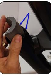
**8.** Adjust the drill torque. Set it as low as possible to start and increase it as needed.
