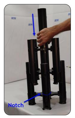
**16.** Maintain pressure to keep the tube engaged in the notch and screw into the hole between the tubes. There is no hole in the center tube, they will form when screwing. Repeat for the 3 others screws of the same level.
