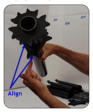
**5.** Take a fishing rod tube and insert the bottom first (1). Slide the bottom part to align with the top part (2).
