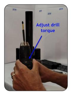
**9.** Take the 1.5 "screws with the stainless-steel washers inserted previously. Point it up and tilt the assembly so the screw stays in place on the drill. Look inside the tube to line up the screw in the hole and screw in until the pieces are thighted together. If necessary, increase the torque.
