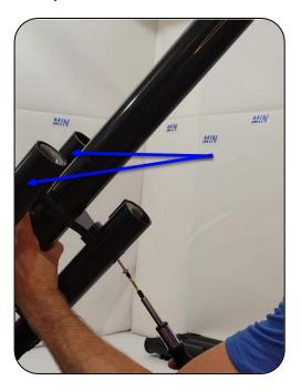
**11.** Insert the top piece (the notch in central the tube) and align.
