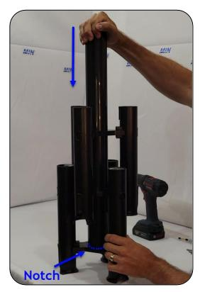
**16.** Maintain pressure to keep the tube engaged in the notch and screw into the hole between the tubes. There is no hole in the center tube, they will form when screwing. Repeat for the 2 other screws of the same level.
